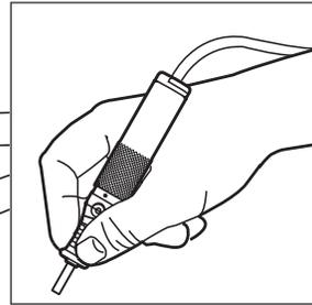
4. **The hammer is usually held like a pencil.** The user should press the hammer tip down firmly on the work **BEFORE** using the foot control to start hammering.
